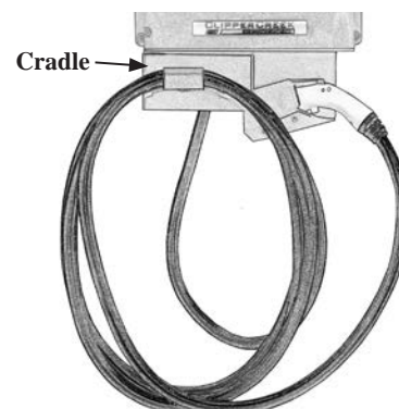
Figure 20: Loosely Wrap Cable Counter Clockwise around the the Cradle
