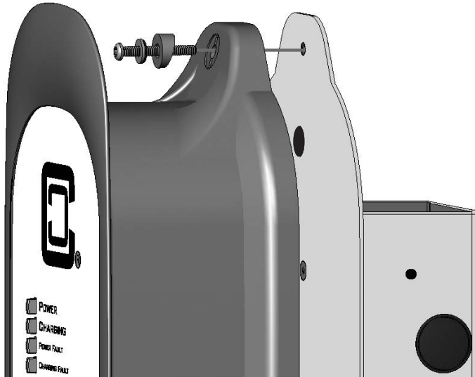
Figure 13: Mounting a Single HCS EVSE, Installing Top Screws FIRST
