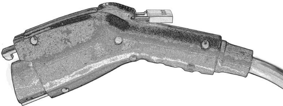
Figure 2. Charge Connector is now secured with Padlock and cannot be removed from vehicle without key.
